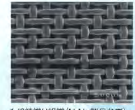
1/2綾織り組織 (N-No製品参考) 1/2 twill weave fabric (referring from N-No. product)
